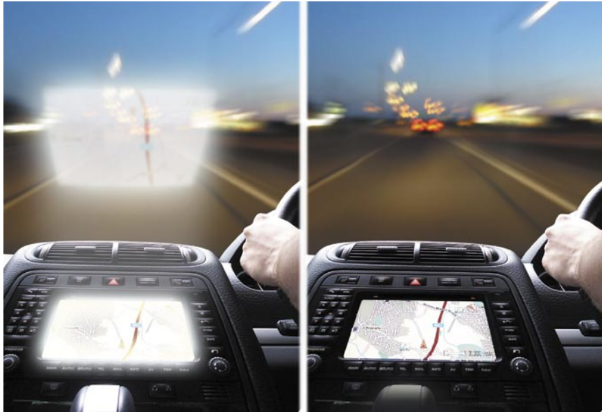
Anti-glare display filter technology combines control of unwanted reflected image with enhanced contrast levels
