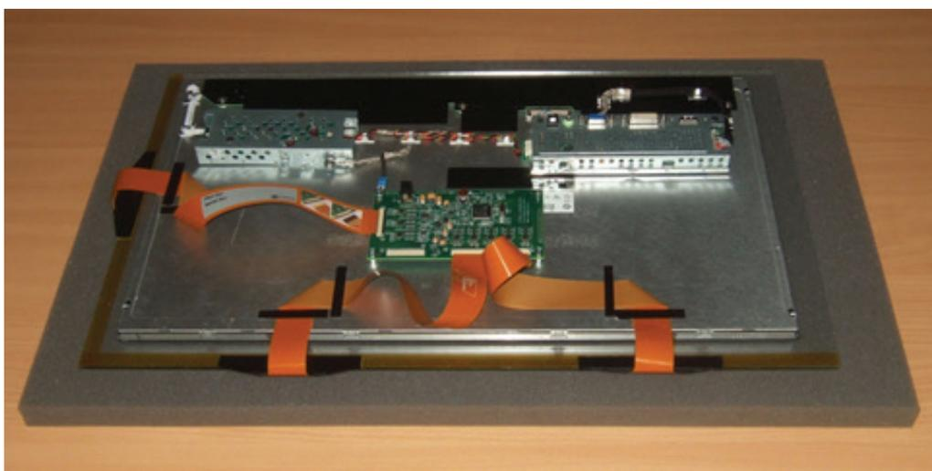
**FIGURE 14** FLEXIBLE CABLES PLUGGED INTO THE CONTROLLER PCB
