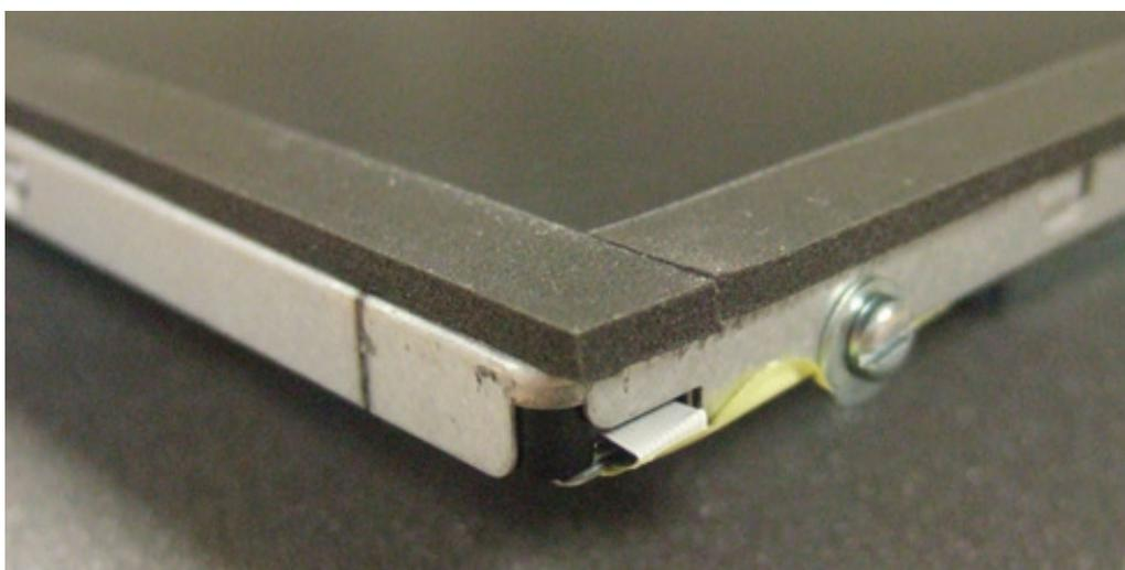
FIGURE 3 GASKET APPLIED TO THE LCD PERIMETER
