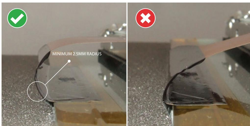
FIGURE 12 FLEXIBLE CABLE BENDING AT SENSOR EDGE
