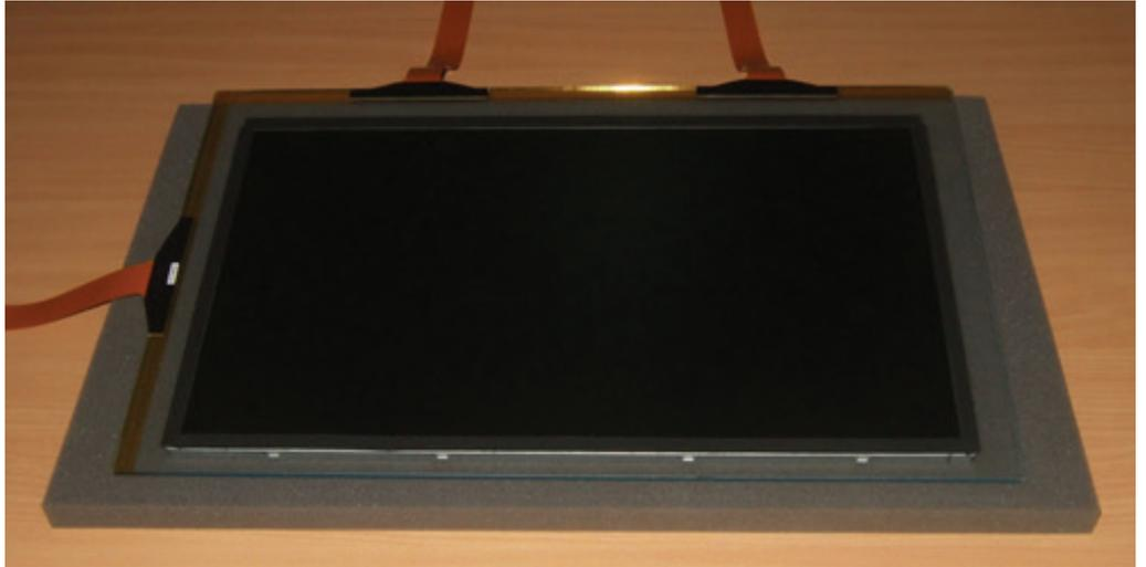
FIGURE 4 SENSOR MOUNTED ONTO LCD WITH GASKET
